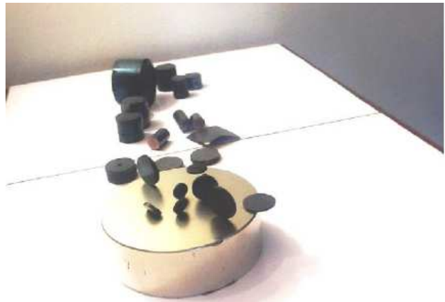
FIG. 20: Side view of some superconductor objects on the same magnet running away from the center or staying upright and at various angles.
