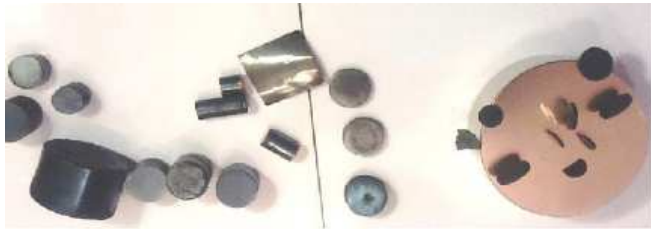
FIG. 19: Top view of some superconductor objects indicating different reflectivity and influence of the magnetic field making them stay upright or sideways, or stick out of the edge.
