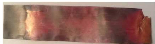
FIG. 22: Results of an experiment of passing 3000\text{A} current via a superconductor tape (left side of the photo) at room temperature of 300\text{K} . The current evidently was passing on the superconductor surface and not along the substrate tape, the positive contact being connected to the bright left part of the tape. The flash burning was with a sharp sound and took about a fraction of a second.
